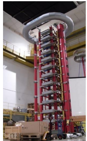
Figure 1 HV impulse generator at TU Dresden
